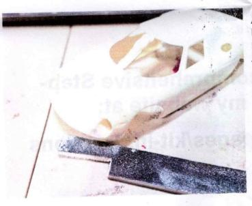
After the superglue dries, use a low grit sanding file to blend the edge between the new resin nose and the plastic kit. YOU DONT have to be perfect with this step, just get it close.
