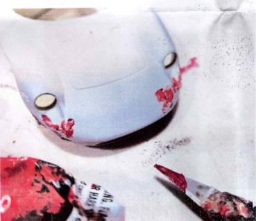
Apply Bondo spot filler putty to any small hole or pin holes or rough areas.
