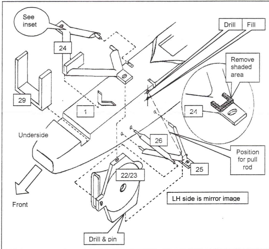
Fit the lower wishbone from under the nose into the slots and shaped location recess. The pins on the rear legs fit into the slots. The top wishbones fit into the holes in the side of the nose cone, the broader legs fits to the foremost holes. Fit the front uprights noting that the air scoop slopes down to the front. It is advisable to 'drill and pin' these joints to reinforce them. Fit the track rods into the holes in the body and the uprights.
