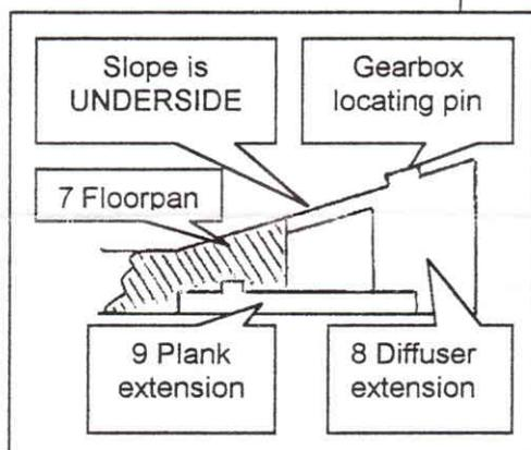
The gearbox locates onto the pin on top of the diffuser extension and butts up against the cross member on the floor pan, (as you look at this part the sloping face is to the underside, see illustration).
