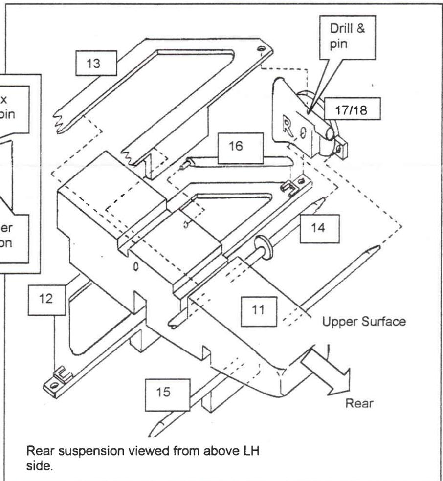
Place the drive shaft axle into the deepest portion of the slot on top of the gearbox; it is then trapped in place by the lip on the top wishbone when fitted in position. The top wishbone fits with the large block to the rear of the car.
